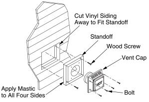
Figure 26 - Installing Vinyl Siding Standoff (Combustible Exterior Wall)
